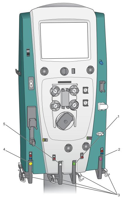
Figure 2:4 Scale components
