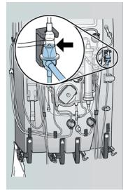
*Figure 4:15* Suggested fluid level in the deaeration chamber.
