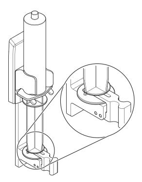
Figure 4:2 B.Braun Perfusor® syringe installation
